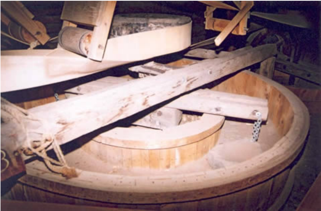
Photograph 4. The arrastra was used to grind the ore to a powder.
