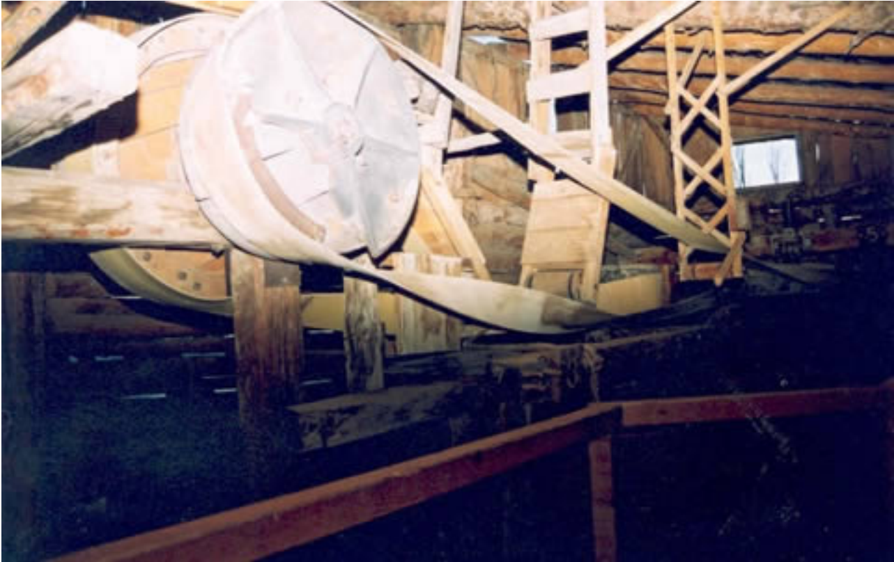
Photograph 2. Conveyor belt used to drive the ore crusher.
