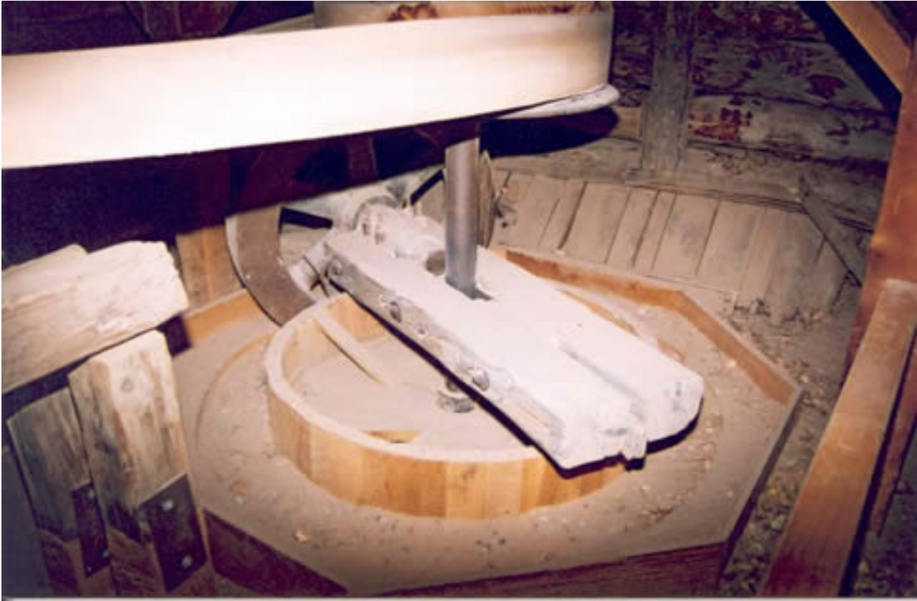
Photograph 3. The ore crusher at Wolverton Mill used a heavy steel wheel.
